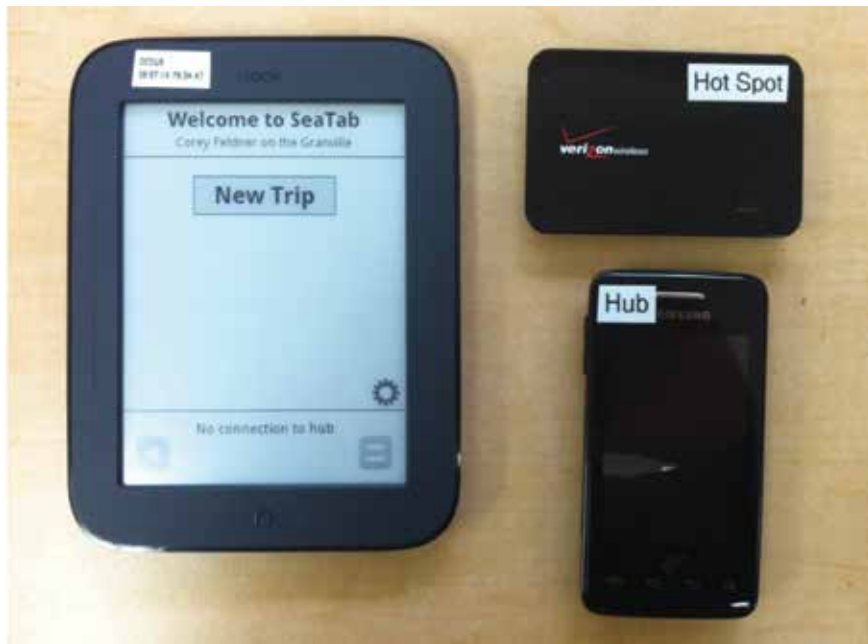
Figure 1. Components of the three-device, at-sea SPT system for small-vessel commercial salmon fishers: Barnes and Noble Nook tablet, MiFi Hotspot, and Samsung Precedent smartphone (Lavrakas et al. 2012). Photo credit: John Lavrakas.
