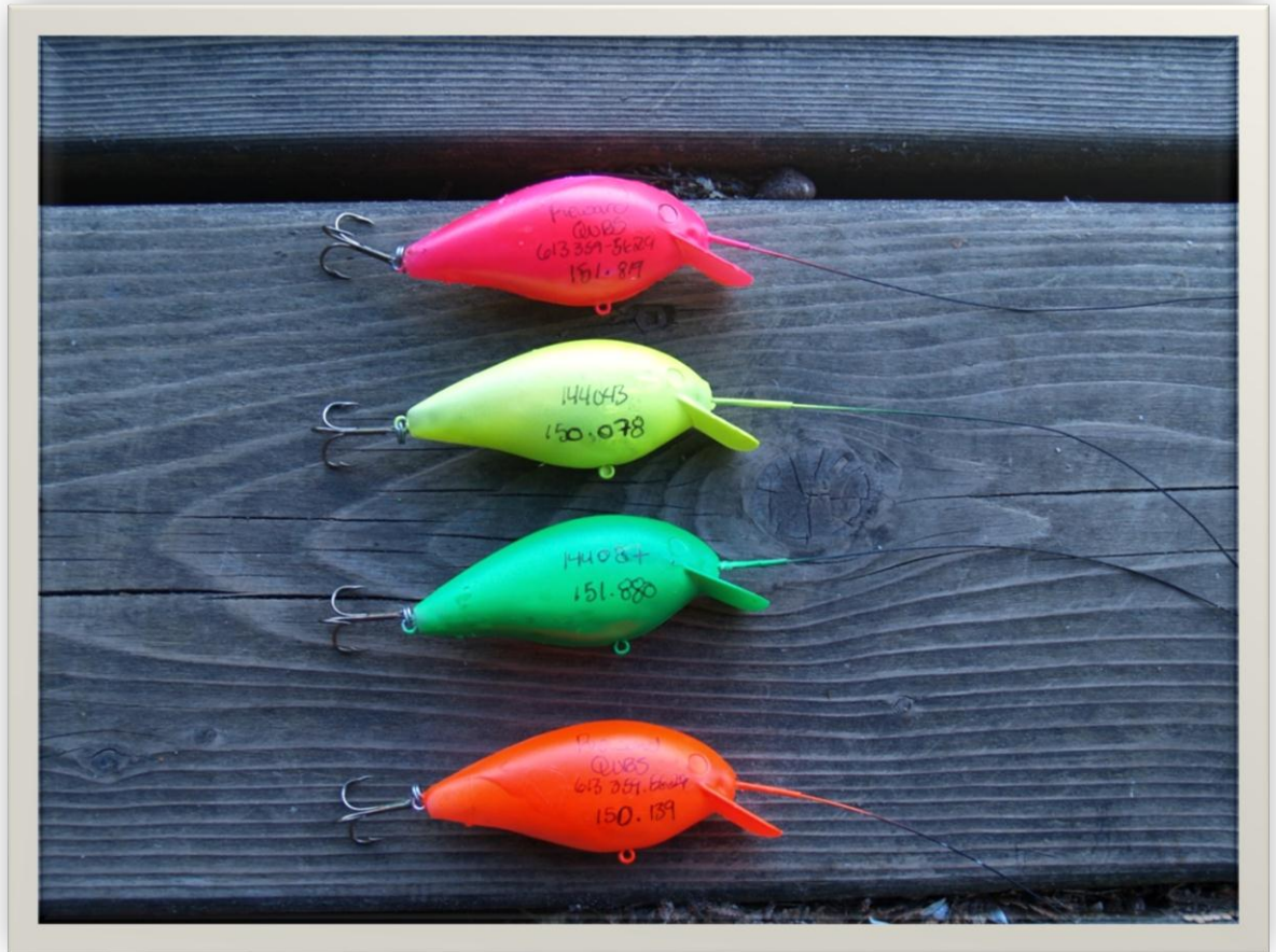
Figure 4-1: Lure treatments included one treble hook at the posterior end of the lure assembly. The transmitter was embedded inside the lure body with the antenna extending out the anterior of the lure: Each colour was assigned to a specific treatment group for ease of recognition once assigned to a fish as well as for locating at a distance on the surface of the lake. Each lure was labelled with transmitter information, research affiliation and contact number. A nominal reward was provided to individuals who returned found lures.
